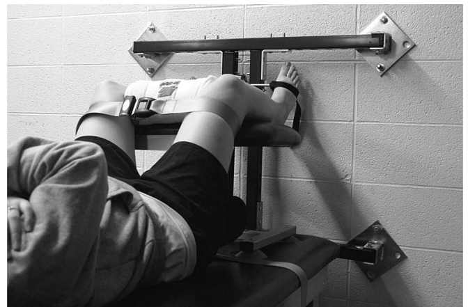
FIGURE 1. Wall-mounted frame with load cell (Sensotec). Subjects were positioned in a supine position on a treatment table with hips and knees flexed, a foam bolster was placed between the knees, and a belt was secured around both legs.
